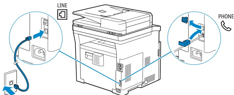
**NOTE:** If the phone communication is serial in your country (such as Germany, Sweden, Denmark, Austria, Belgium, Italy, France and Switzerland), and you are supplied with a yellow terminator, insert the yellow terminator into the phone connector.
